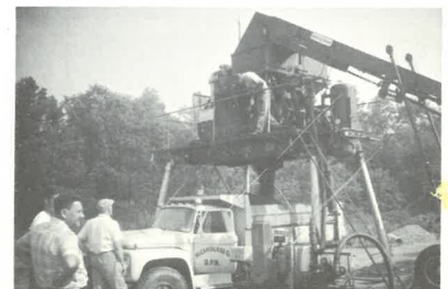
Portable Asphalt Mixing Plant, to 800 Tons per Day
